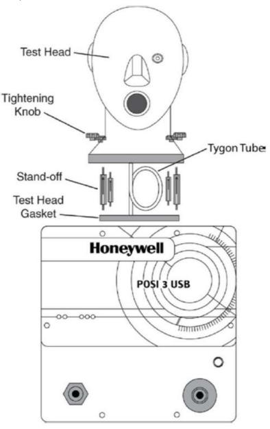
3. Connect the Tygon™ tube from the hose barb on the bottom of the head to the hose barb at the bottom front of
