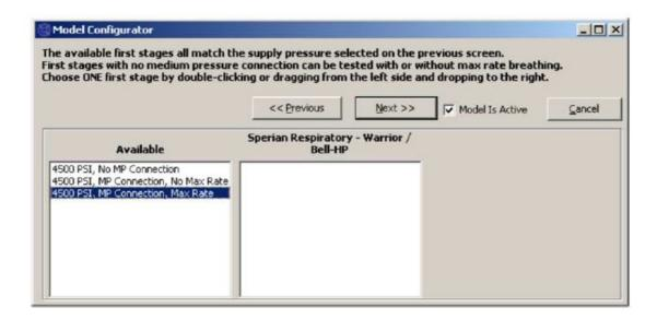
**Note:** "MP" stands for Medium Pressure. For models with a Medium Pressure connection in the Standard Software, the medium pressure readings will be shown on appropriate tests. The Standard Software does not contain tolerances for the medium pressure tests, so there will be no indication whether the medium pressure portion of the tests passes or fails.
