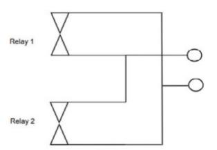
Normally Closed Contacts (as labelled on the module) Configuration 2 The environmental conditions that the Searchline Excel Plus & Edge is designed to operate within are listed
