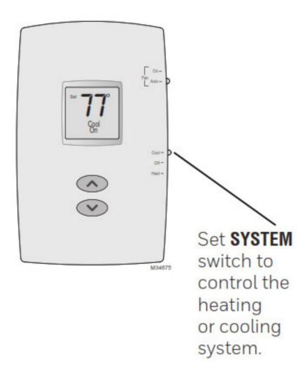
The SYSTEM switch can be set to control your heating or cooling system, depending on the season.
