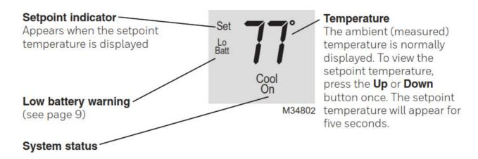
**Cool on**: Cooling system is on. **Heat on**: Heating system is on.
