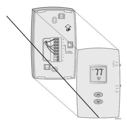
Pull at the bottom to remove the thermostat from wallplate.
