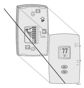
Pull at the bottom to remove the thermostat from the wallplate.
