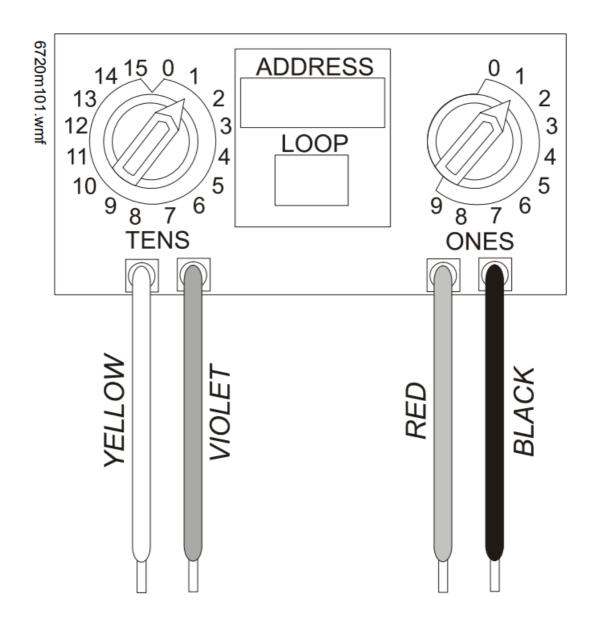
The NMM-100P(A) Mini Monitor Module can be installed in a single-gang junction directly behind the monitored unit. Its small size and light weight allow it to be installed without rigid mounting. The NMM-100P(A) is intended for use in intelligent, two-wire systems where the individual address of each module is selected using rotary switches.
