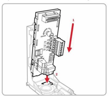
9. Tighten the retaining screw to secure the power PCB module.
