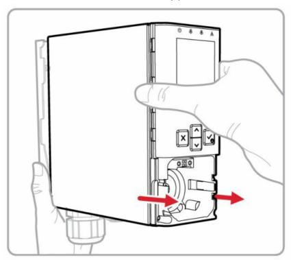
3. Unscrew the retaining screws located at the base module, and then, remove the back plane PCB module.
