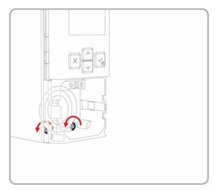
2. Remove the main module by pulling it forwards off the base module. At this time, hold the cable gland in the base module with one hand, and with the other hand, carefully pull the main module.
