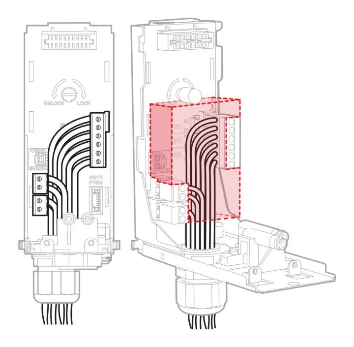
Note: Wiring should be executed within the red area.
