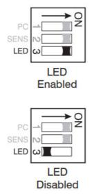
After applying power to the sensor, it will warm up for up to three minutes, and then the LED will temporarily remain enabled for a 10-minute walk-test period. After 10 minutes, the LED will automatically switch to disabled. To restart the 10-minute walk-test mode, switch S3 ON, and then OFF again
