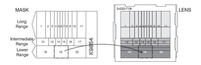
Use Lens Mask K9855 to mask Long, Intermediate and Lower Range segments on the High Security/Non-Pet Immune Lens (P/N 5-532-477, included).
