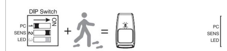
Low Sensitivity: 2-4 Steps (High Sensitivity and Pulse Count 2) Note: This is the recommended setting for applications with pets up to 18 kg (40 lb) when used with the Pet Immune Lens.
