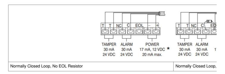
**Note:** EOL = End of Line supervised resistor / spare terminal block. \*For UL voltage, see Specifications Section. **Select the appropriate lens\* for the installation. If necessary, mask segments as required.** (Refer to the Masking the Lens section.)
