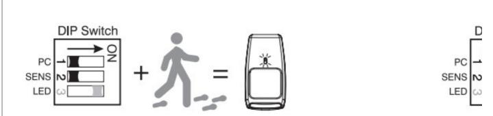
Lowest Sensitivity: 3-5 Steps (Low Sensitivity and Pulse Count 2) Note: This is the recommended setting for applica to 36 kg (80 lb) when used with the Pet Immune Lens, or Harsh environments.
