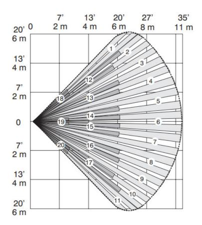
**Note:** Detection may occur beyond the distance ide ViewHigh Security/Non-Pet illustrated. A walk test is required after mounting to ensure proper detection.
