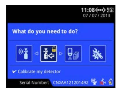
Bump test is a procedure that confirms a detector's ability to respond to target gases by exposing the detector to gas concentrations that exceed its alarm setpoints.
