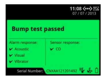
When the calibration is successful, LCD screen background changes to green and Calibration passed is displayed. Alarm response and sensor response test items are checked. Press to return to IntelliDoX user menu.
