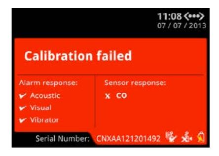
When the bump test fails, LCD screen background changes to red and Bump test failed message is displayed. Failed alarm response and/or sensor response test items are marked with . If the AutoCal on Failed Bump is set using PC configuration software, calibration automatically begins.
