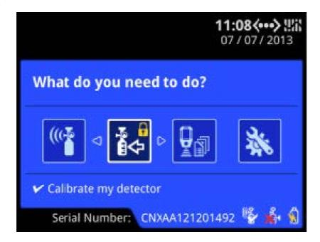
AutoCal on Overdue Sensors is set using PC configuration software and sensors are overdue, then calibration starts automatically once IntelliDoX recognizes the detector.
