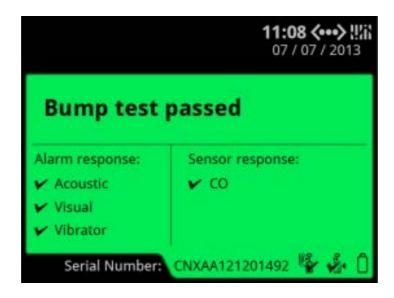
When the bump test is successful, LCD screen background changes to green and Bump test passed message is displayed. Alarm response and sensor response test items are checked. Press to return to IntelliDoX user menu.
