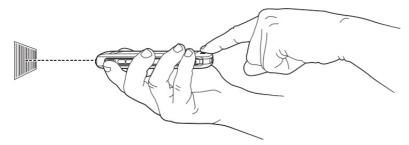
On a successful scan, the terminal beeps twice and "configuration received" appears under the Barcode option on the screen.
