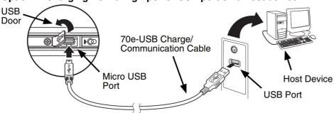
**Note:** Charging the battery through a USB port takes more time than direct AC adapter charging. USB charging will not take place if the terminal is drawing more current than supplied by the USB port. Refer to the user's guide for additional information.
