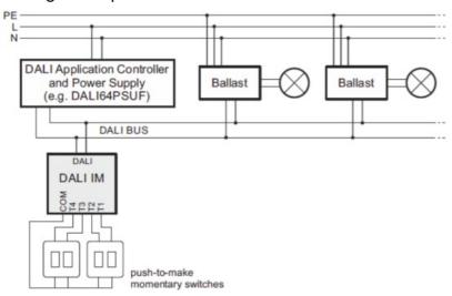
⚠ Warning: The DALI bus is not classified as SELV. The same procedures and safeguards must be applied as when working with mains voltage.
