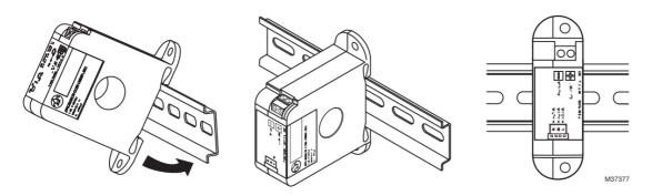
Fig. 1. Sensor Placed on Rail.
