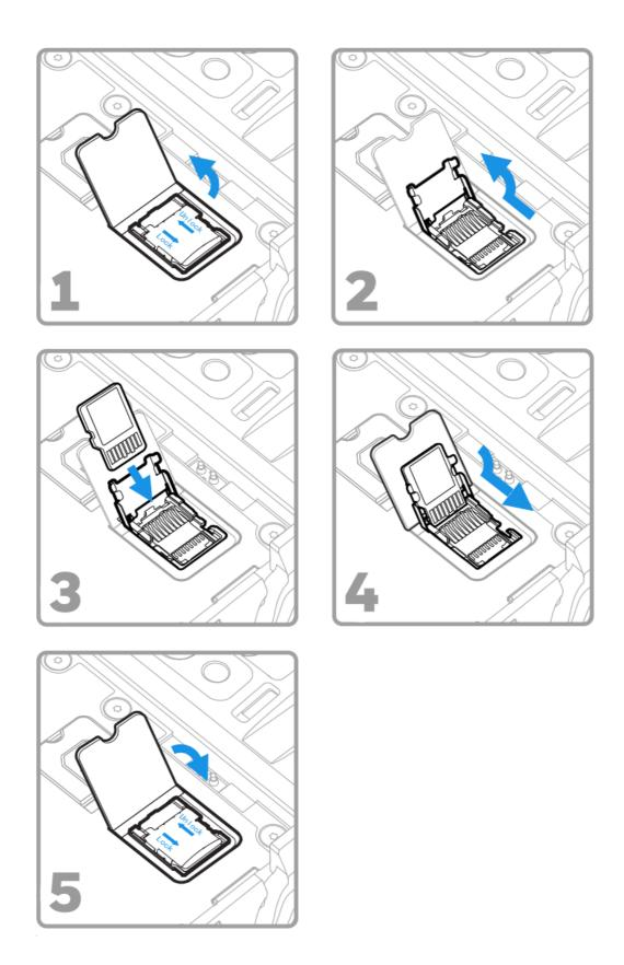
**Note:** Always power off the computer and remove the battery before attempting to install or remove a card.
