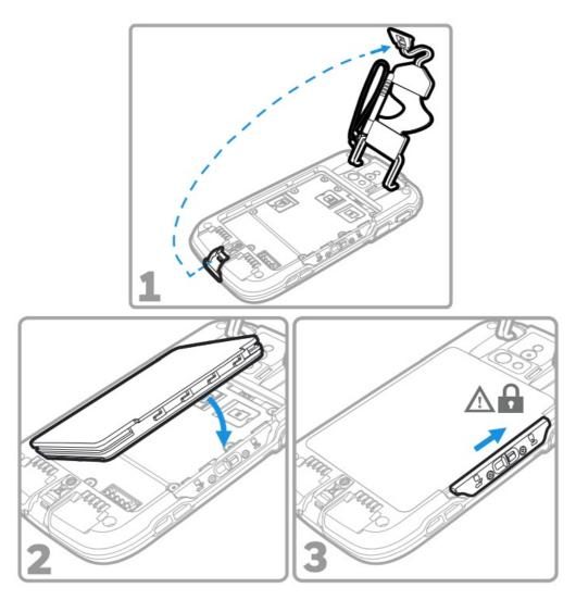
Ensure all components are dry prior to placing the battery in the computer. Mating wet components may cause damage not covered by the warranty.
