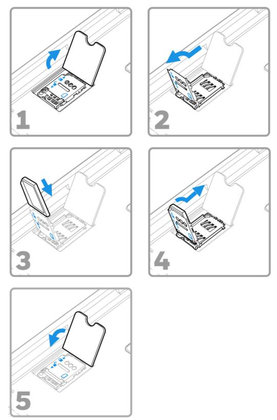
**Note:** Always power off the computer and remove the battery before attempting to install or remove a card.
