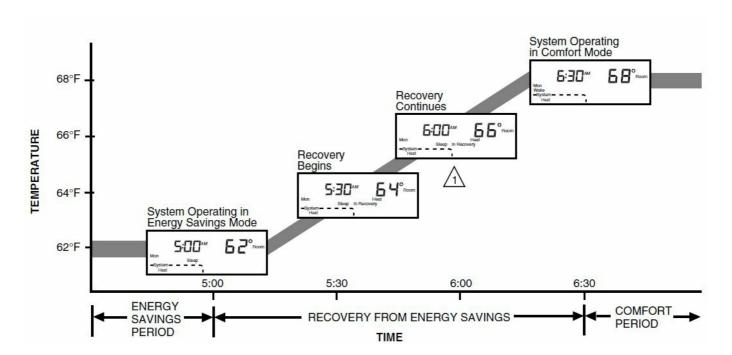
THE THERMOSTAT USES THE SAME SCHEME TO RETURN TO LOWER COMFORT TEMPERATURE DURING THE COOLING SEASON.
