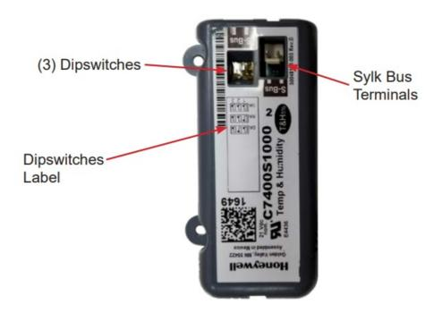
The economizer comes standard with a C7400S outdoor enthalpy factory mounted in the outdoor air stream, and is factory wired to the W7220 Logic Module. A second C7400S enthalpy sensor can be added to measure the return air enthalpy and provide a dual enthalpy strategy. The C7400S sensor is shown above in Figure 1.
