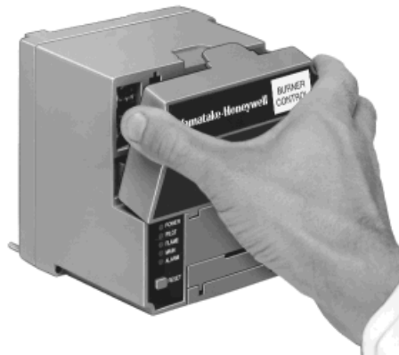
Fig. 12. Dust Cover mounting.
