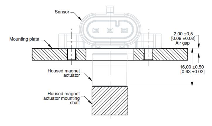
FIGURE 2. MOUNTING DIMENSIONS (FOR REFERENCE ONLY: MM [IN].)
