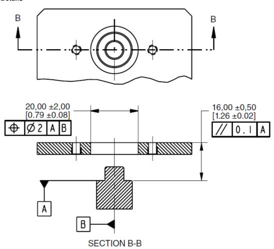
**Sensor and Housed Magnet Actuator on Mounting Plate**
