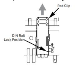
3. Hold the controller as shown in image below and mount the controller onto the DIN rail.
