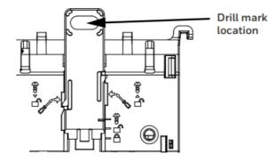
3. Remove the controller from the wall and drill four holes at the marked locations.
