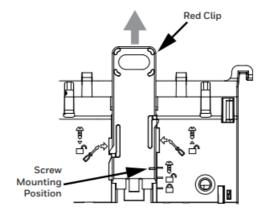
2. Hold the controller along the wall and mark drilling locations through the screw red clip slots, as shown in the figure below.
