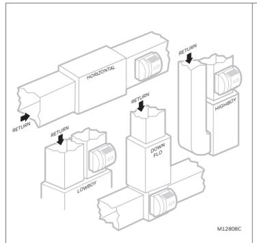
Fig. 1. Typical humidifier installation locations.
