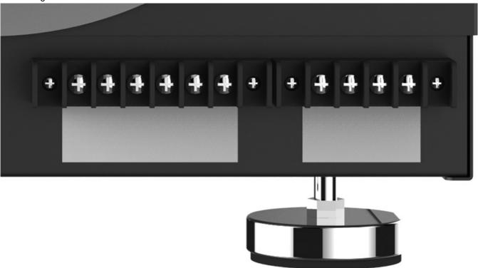
The six terminals for the left hand terminal block are: FLOAT (2): External low-voltage water sensor or float switch
