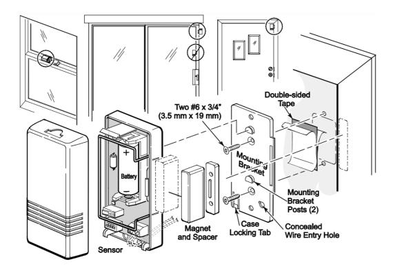
After enrolling and before permanently mounting, conduct Go/No Go tests (see the control's instructions) to verify adequate signal strength. Reorient or relocate the device if necessary.
