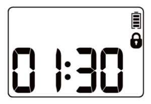
Make sure the timer dial is at the "AUTO" position. Press and hold the \*-" button for 5 seconds until " appears on the screen. If you want to cancel the child lock setting, please press and hold \*-" again for 5.
