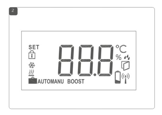
Set/actual temperature Humidity Warning about condensation Open window symbol Battery symbol (q) Radio transmission **Boost function** BOOST Manual operation MANU Automatic mode AUTO Holiday mode 222 Heat \* Cool 園 Operating lock SET Setpoint temperature
