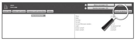
• To activate pair mode of the CCU3, click on the desired pairing window (e.g. "Add HmIP device"). The pair mode of the Central Control Unit will be activated. An information box shows how much pairing time remains.
