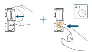
• Release the system button (A) briefly and then hold the system button (A) down again until the orange flashes are replaced by a green light.
