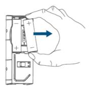
• Place the two new 1.5 V LR6/Mignon/AA batteries in the battery compartment (F) by the polarity markings.
