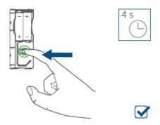
• Release the system button (A) again to complete restoring the factory settings.
