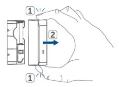
• When not mounted, the cover cap (B) can be removed by pressing the upper and lower sides with one hand. At the same time, take hold of the rib of the electronics unit (G) on the rear side of the HmIP-ESI with your other hand and pull it out of the cover.
