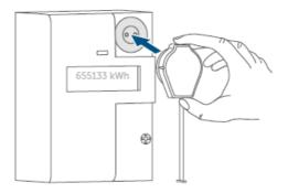
The integrated magnet ensures it remains in place. With standard-com-pliant interfaces, the cable is routed downwards.
