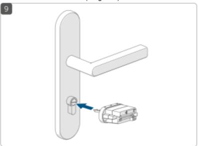
• Attach the desired cover (B) (white or silver) to the door lock sensor (s. figure 10).
