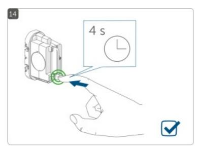
• Release the system button to finish the procedure. The device will perform a restart.
