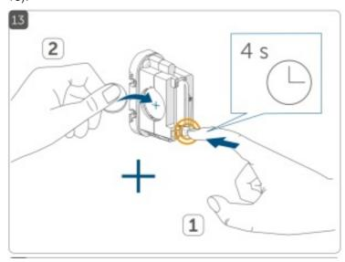
• Release the system button briefly and then press and hold the system button again until the orange flashing changes to a green light (s. figure 14).
