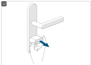
Note: The cover can be removed easily if the key is not in the neutral position.
