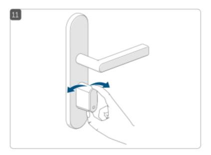
If the door lock sensor will be used in another lock/another door or the sensor was removed from the lock, you need to repeat the process once of inserting the sensor in the lock and then completely locking and unlocking (with the lock latch).
