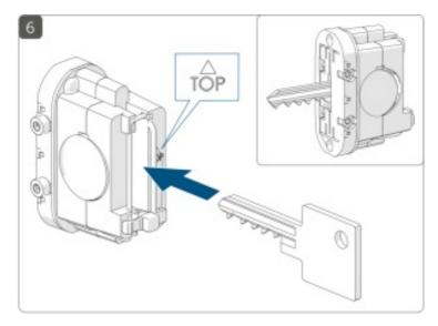
• Retighten the screws so that the door lock sensor fits securely on the key (s. figure 7).
