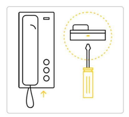
The housing of the intercom system is usually clipped or screwed on. First remove the screws. If the housing is clipped on, press the enclosed screwdriver carefully into the hole on the bottom of the housing and lift the housing up. You can simply leave the handset hanging down.
