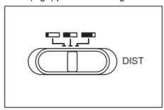
The higher the "DIST" setting (Distance), the greater the possibility of false triggering.
