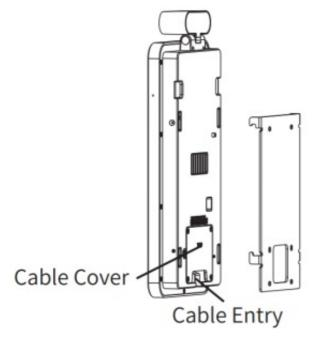
4. Hang the device onto the bracket hook and then tighten the screws.
