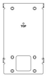
2. Install the gang box on the wall. Then use two screws to secure the bracket on the gang box. Secure the bracket onto the wall with 4 screws.
