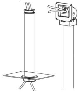
4. Tighten the screw with a L-shaped screwdriver.
