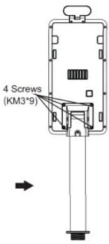
8. Loosen the screws to adjust the angle of the device.
