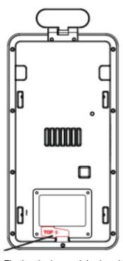
7. Fix the device and the bracket with four screws.
