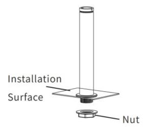
3. Install the pole and then tighten the nut.
