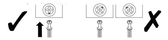
**EN\_Quickfit** head should be in the centre of the cam lock when the two panels are joined.
