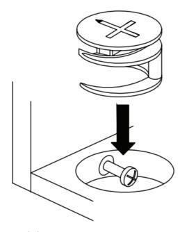
EN **Turn** cam lock clockwise to tighten.
