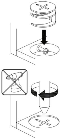
• Turn the cam lock clockwise to tighten.
