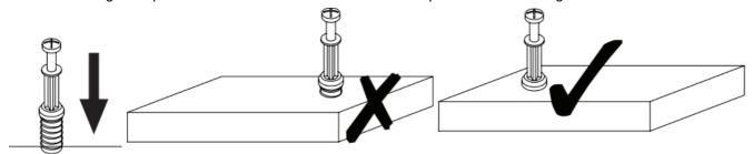
• CAM LOCK: When fitting the cam lock, ensure the starting position is correct before you insert the connecting quickfit.
