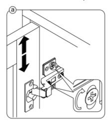
• To adjust the gap from the door to the main frame turn the screw clockwise or anti-clockwise as needed.
