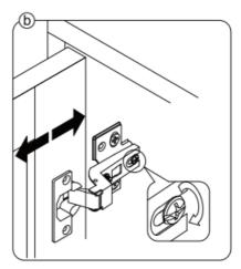
• To adjust the door laterally adjust the screw as shown by turning clockwise or anti-clockwise.
