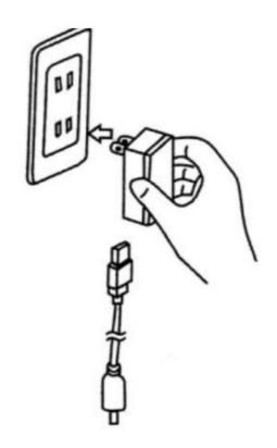
**Charging:** Please use the power adapter correctly. Charge the lamp 5V-2A
