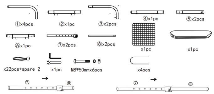
**Tip:** Tube 8 is in tube 7, pull tube 8 out from tube 7 when assemble the product frame.
