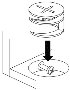
Turn cam lock clockwise to tighten.
