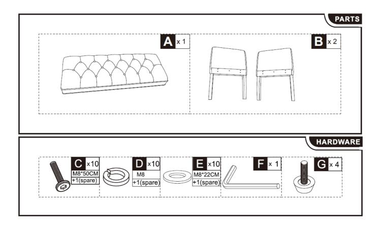
Do not confuse similar screws. Do not tighten bolts fully until all parts are connected!
