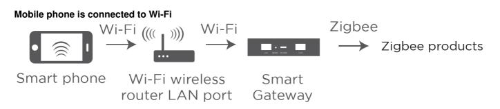
Ensure that the smart phone is within the same Wi-Fi network of the Smart Gateway to ensure an effective connection between the smart phone and the Smart Gateway.
