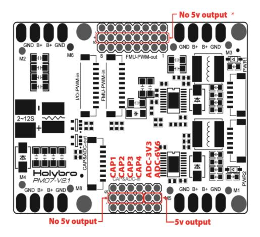
• **Note:** If using a plane or rover, the 8 pin power (+) rail of FMU PWM-OUT will need to be separately powered in order to drive servos for rudders, elevons etc. To do this, the power rail needs to be connected to a BEC equipped ESC or a standalone 5V BEC or a 2S LiPo battery. Be careful with the voltage of servo you are going to use here.
