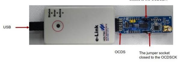
Connects to the USB port for programming using the HT-IDE3000. If problems are encountered, refer to the HT-IDE3000 User's Guide.
