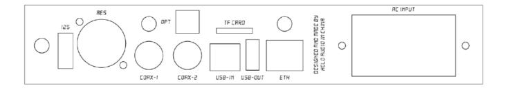
From left to right (top to bottom) interfaces are: optical fiber, system TF card holder\*, 2 1 s\*, AES, coaxial 7 \*, coaxial 2\*, USB input, USB output, network port, AC power input
