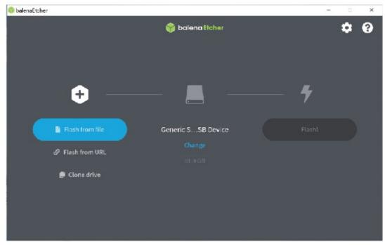
• Select the desired system image (.img file) in the BalenaEtcher-Portable sofuNare under "Flash fTDm file", select the corresponding TF drive letter under "Select target", and then select "Flash!" to start writing to the system. A dialog box will appear asking if you are sure, select "Yes"
