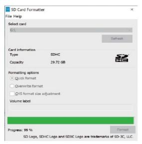
After the formatting is completed, drive capacity and storage space can be seen; click "OK" to close the software.
