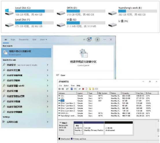
In addition, you can use the SD Card Formatter tool to format the TF card. Proceed as follows: Run SD Card Formatter and select the TF card to be formatted. !!! Carefully check the drive letter that needs to be formatted to avoid the tragedy of formatting other disks!!!
