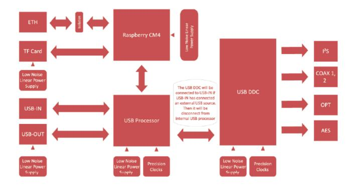
When the USB-IN is effectively connected, the USB DDC will be connected to the USB-IN and disconnected from the USB processor; 12s, COAX-7, COAX-2, OPT, AES will simultaneously output the audio signal from the USB-IN.
