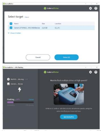
BalenaEtcher-Portable sofuNare under "Flash fTDm file", select the corresponding TF drive letter under "Select target", and then select "Flash!" to start writing to the system. A dialog box will appear asking if you are sure, select "Yes"
