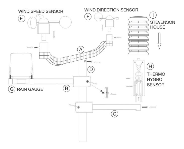
Fit the Wind Speed Sensor (E) to the end of the 'U-Shaped' plastic bracket (A)
