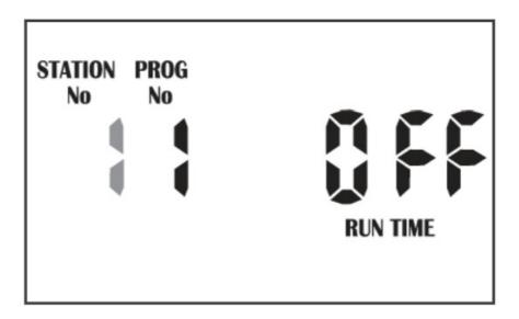
STATION No. 1 will be flashing labelled as OFF, as shown above, meaning it has no RUN TIME programmed in it
