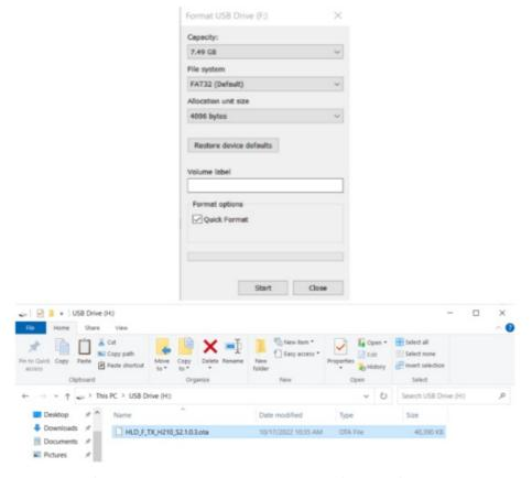
2. Insert the USB flash disk into the wireless monitor's Type-C port will the monitor enter the updating status automatically after 1 mins around. Then just waiting for the updating completion
