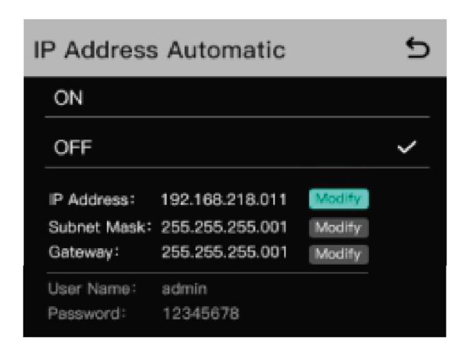
• Use a network cable to connect the hub to a computer via the RJ45 interface and set the IP address of the computer as 192.168.218.XXX. The default IP address of the hub is 192.168.218.10.
