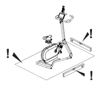
**CAUTION!** The training machine must be positioned on a horizontal, stable surface. Place suitable cushioning material underneath it for shock absorption and to stop it from slipping (rubber mats or similar). The safety distance around the bike must be at least 1 metre larger than the area in which you are exercising.
