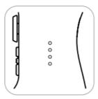
4 LED lights on: 100% 3 LED lights on: 75% 2 LED lights on: 50% 1 LED light on: 25%
