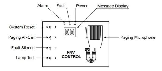
The Fault LED will flash when a fault has occurred in the system and the audible trouble Annunciator will sound. The specific fault will be displayed on the MMC and, if thefault is associated with a switch, on the SLC (Switch/LED Card) as well.
