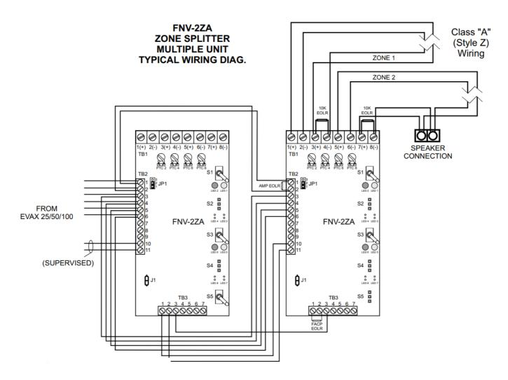
Additional units may be daisy chained in the same fashion. Insure that EOLRs are installed at last Zone Splitter to maintain supervision.
