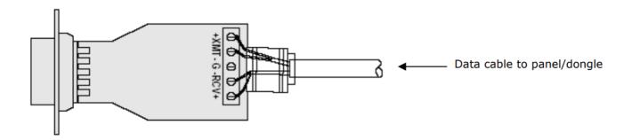
The data cable should be secured to the converter using the cable clamp and routed such that it is not likely to be
