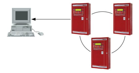
The FireNET graphix system can be connected to a single fire alarm control panel or a network of control panels by up to 3,900 feet (1,200 metres) of suitable RS-485 data cable.
