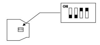
Switch 1, 2 OFF Switch 3, 4 ON
