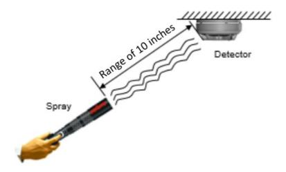
Test with Smoke Sabre aerosol cans or the Testifier 1000/1001 or 2000/2001 with TS3 smoke capsules.
