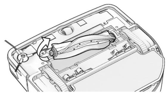
3. Use the cleaning tool to cut loose the tangled hair and debris to clean the brush roll, rinse then dry when needed.
