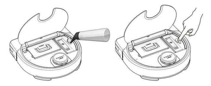
\*, DO NOT use any other detergent or liquid to prevent blockage of the pipes and the spray nozzles.
