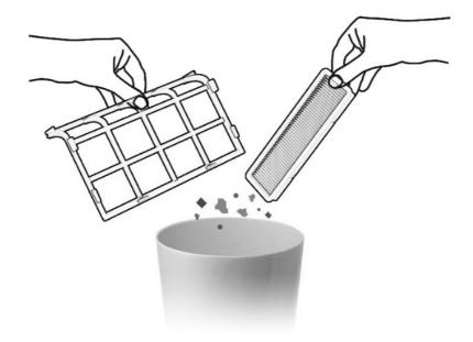
2. Rinse the filters if necessary. Do NOT rub the filters or use high-pressure water. Be sure to leave the filters to dry thoroughly before reinstalling them.
