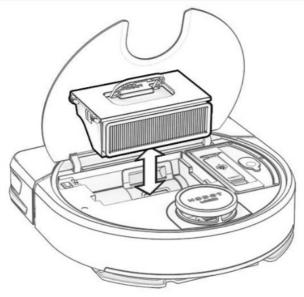
2. Remove the screen filter and empty the trash bin.
