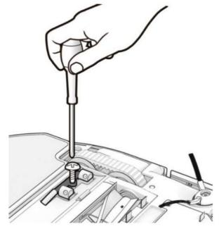
2. Replace the old nozzles with new ones, then reinstall the nozzles.
