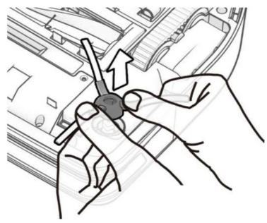
2. If necessary, rinse the side brush with warm water to clean the dirt off and restore it to its original shape.
