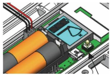
3. Open the sensor node door and install the rechargeable batteries. Press the button on the sensor node for 3 seconds.
