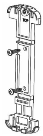
2. To install the bracket onto a wall, use the two long screws included in the package. Screw the bracket to a wall using the two holes on the mid-section of the bracket.
