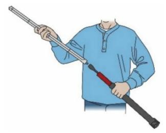
3. Screw the pilot rod into the slide hammer. Use two adjustable wrenches to make sure the threads are tight between the slide hammer and pilot rod.
