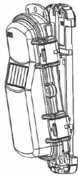
4. Insert the bottom of the sensor node into the retaining clips on the bottom of the bracket then press the top of the sensor node into the clips at the top of the bracket.
