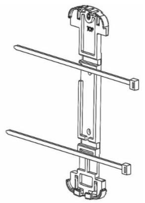
3. To install the bracket onto a pole, slip a cable tie through each of the channels on the bracket and fasten the tie around the pole.
