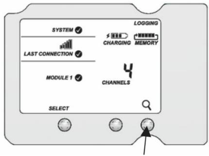
2. Press the Search button. The magnifying glass icon blinks while the station is in search mode waiting for sensor nodes to join the network.
