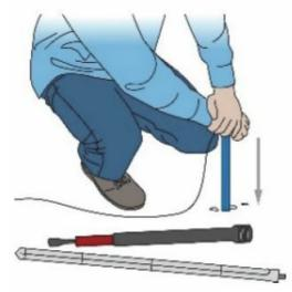
• **Important:** Do not use a hammer or other tools to push in the sensor because they may damage the sensor.
