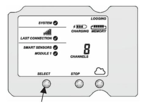
1. Press the Select button on the station to switch to the module with the manager (module 2 on RX2105 or RX2106 stations).
