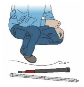
8. Pack the soil around the top of the sensor to prevent water from entering the hole. The sensor should be completely covered with soil and only the sensor cable visible.
