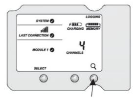
3. Open the sensor node door and install the rechargeable batteries. Press the button on the sensor node for 3 seconds.
