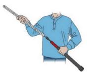
5. Once the pilot rod reaches the desired depth, extract the pilot rod by using the slide hammer in reverse, lifting it rapidly to hammer upwards.
