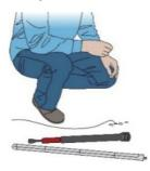
8. Pack the soil around the top of the sensor to prevent water from entering the hole. The sensor should be completely covered with soil and only the sensor cable visible.
