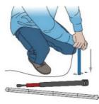
7. Insert the sensor probe into the hole, pressing it in as far as possible by hand. Pour a bit of water around the probe at the top of the hole if the soil is very tightly packed to help it slide more smoothly into the hole.
