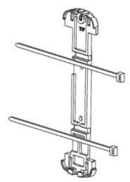
4. Insert the bottom of the sensor node into the retaining clips on the bottom of the bracket then press the top of the sensor node into the clips at the top of the bracket.
